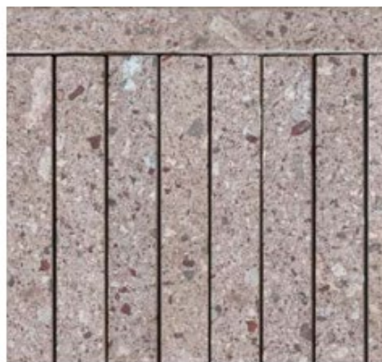
B-Plinth stone Granite, palette to connect the light colour render with existing pavers
